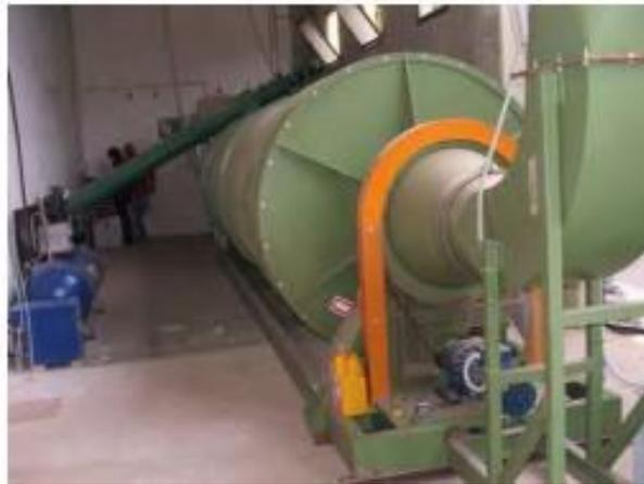
Figure 11 E Example of rotary dryer to be used in the drying process.
