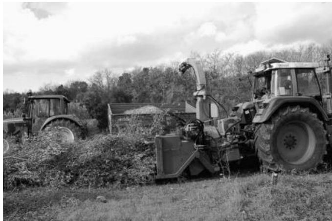
**Figure 9 - Tractor-mounted machine while harvesting olive pruning residues. The high-tipping bin is not installed here and biomass is blown onto a towed trailer (Source:[11])**
