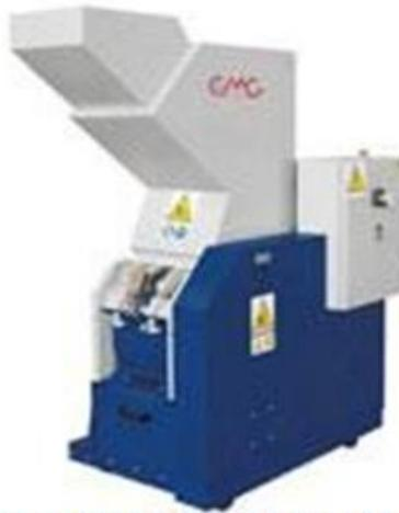
Figure 10 - Granulator–Size reduction solution used to perform preliminary tests
