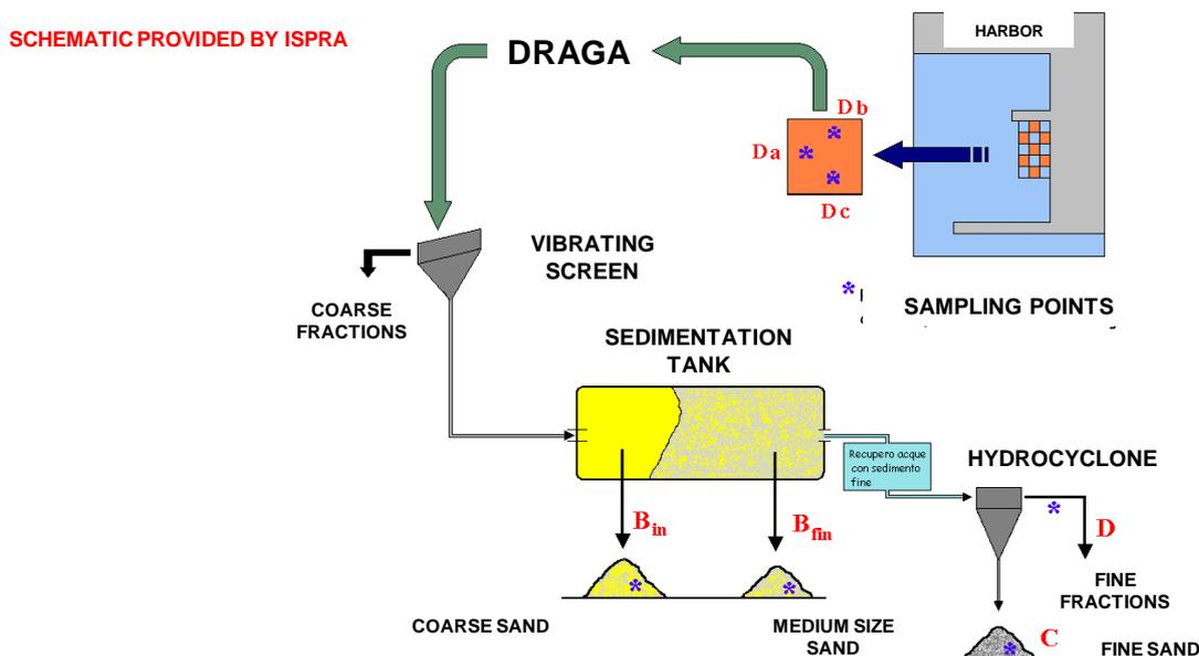
Figure 1 – Schematic of the ISPRA pilot plant in Piombino
